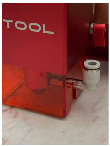
FIG. 12. The supplied air intake connector screws directly into a threaded opening in the laser nozzle.
