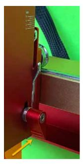
FIG. 7. The release lever on the right side of the laser module is used to set the position of the laser height (z-axis) for cutting, using the increments inscribed in white on on the upper edge.
