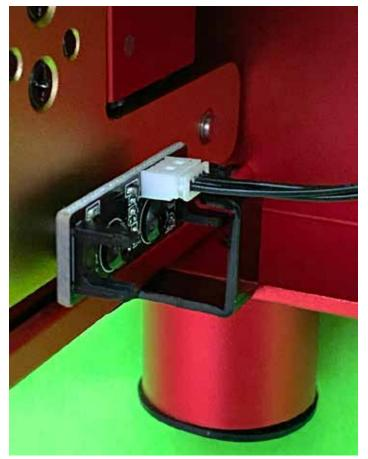
FIG. 11. xTool uses an advanced design, long-lasting electronic limit switch, which is superior to a mechanical roller lever arm.
