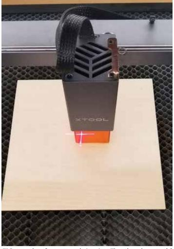
FIG. 8 crosshair-fitting-material\_480x480. The red crosshairs simplify the placement of the laser head with brightly illuminated reference lines.
